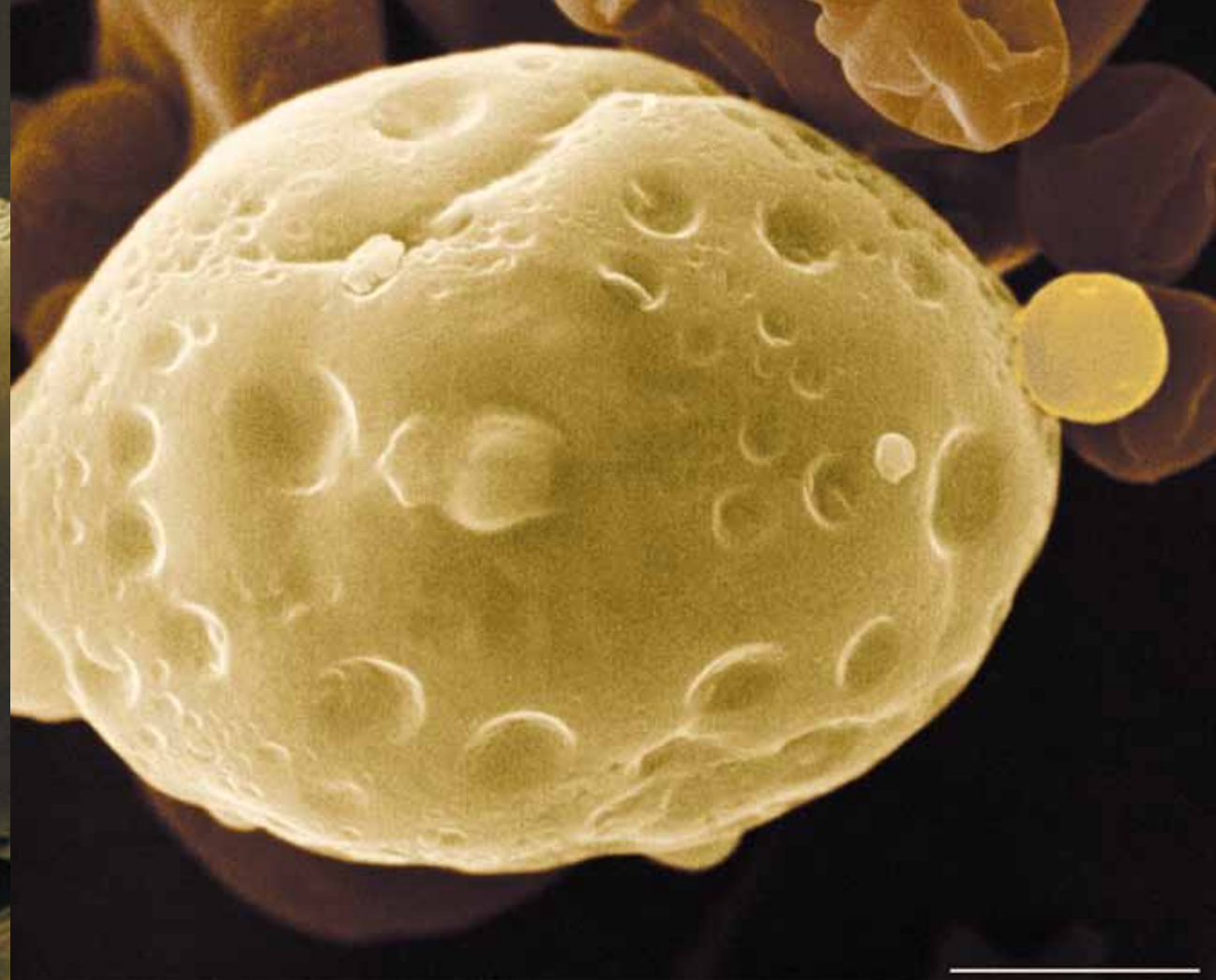
Fig. 21. Some spray-dried milk particles have dimples on their surfaces. Bar: 10 \mu\text{m} .
