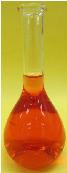
Figure 4-18: Volumetric flask filled to calibration line with water. Colouring was added to the water for visual clarity.
