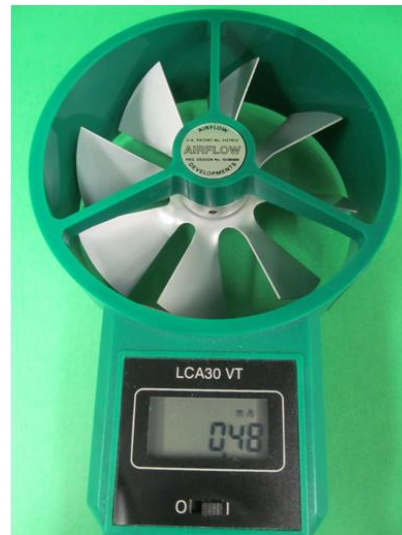
Figure 8-25: A linear air velocity of 0.48 m/s is indicated on this vaned anemometer.
