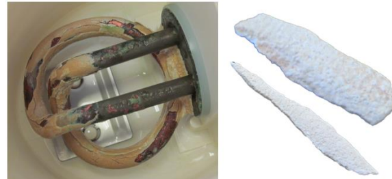
Figure 6-42: Partially cleaned coils in kettle and pieces of calcium carbonate removed from coils.
