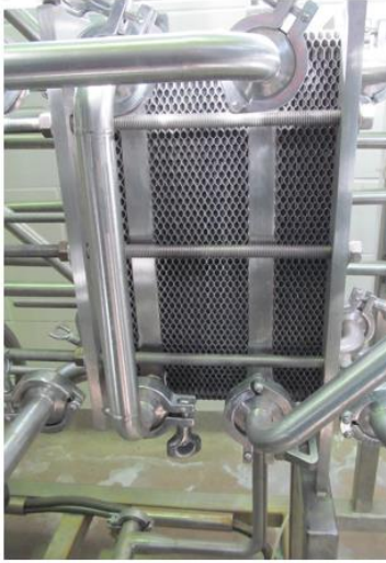
Figure 3-5: Plate heat exchangers have improved thermal processing of liquid products.
