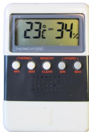
Figure 8-24: This electronic hygrometer indicates that the relative humidity of the air at 23°C is 34% and that the air is considered “dry”.
