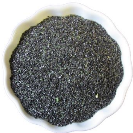
Figure 10-25: Activated carbon from the cartridge of a home water treatment system.
