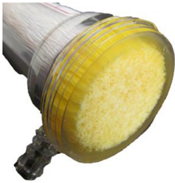
Figure 10-5: An end view of the membrane cartridge showing the openings of the potted hollow fibres.
