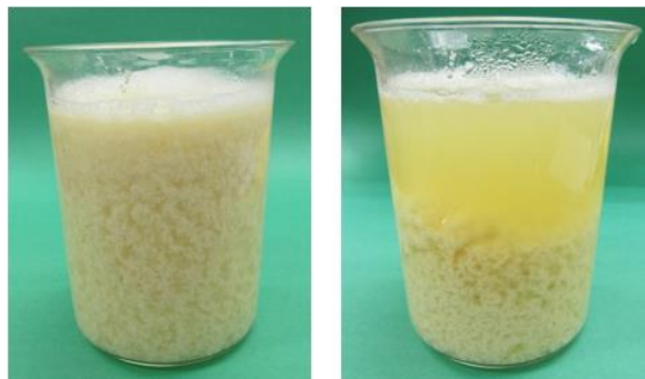
Figure 10-27: Protein curd formed in soy milk (left photo) will settle (right photo) and can be recovered by filtration.
