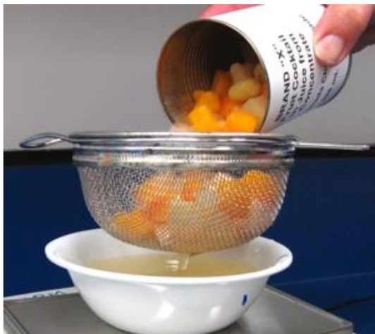
Figure 10-1: A sieve (or strainer) is an example of separating mixtures of solids and liquids on the basis of particle size.
