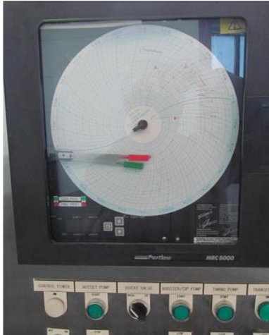
Figure 6-33: Circular recording chart for a thermal processing unit.
