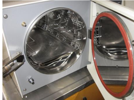
Figure 5-14: Autoclave used for sterilizing laboratory equipment. Closed in upper photo and open in lower photo.
