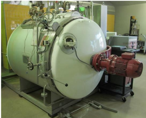
Figure 6-4: Small retort unit for studying thermal processing of canned food products. (Red motor assembly powers fan to enhance steam circulation inside retort).
