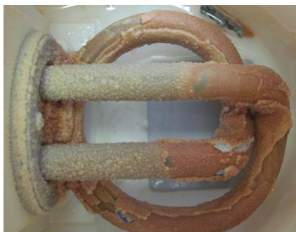
Figure 6-41: Calcium carbonate (limestone) deposits on heating coils in kettle.
