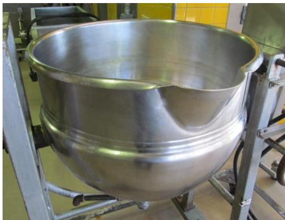
Figure 6-24: Jacketed kettle in pilot plant facility.
