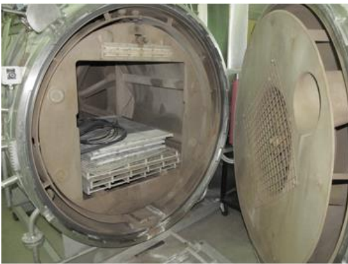
Figure 6-5: Interior of small retort unit for studying thermal processing of canned food products. (Circulating fan is housed in door).
