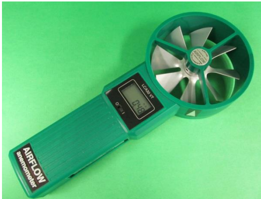
Figure 5-15: A hand-held anemometer for measuring air velocities
